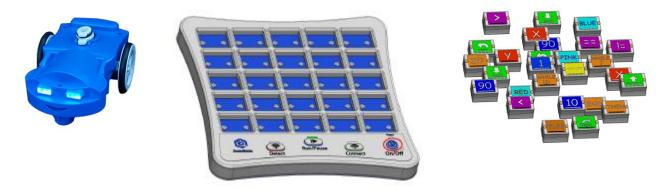
Users place Qubes in a logical mathematical sequence to create a movement pattern for the QuestBot. Sequences can include linear movement, circles, angles, functions, there is no limit! The QuestController hold the Qubes in a 5x5 grid, and the code is read on the QuestController from left to right, top to bottom, just like reading a book.
